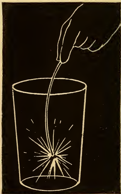
FIG. 22. WATCHSPRING BURNING IN JAR OF OXYGEN
